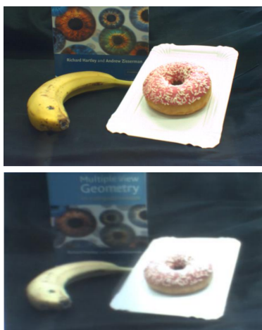
(a) Color distortion is a common problem when using optical see-through glasses (image taken from [48])
