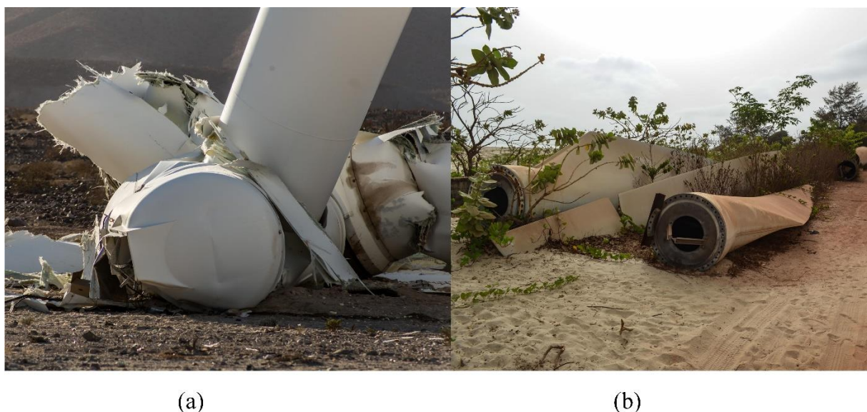
Figure 1. (a) An abandoned collapsed wind turbine, (b) End-of-life wind turbine blade dump fills on the roadside: Reproduced from Ref. [6,7] with permission.
