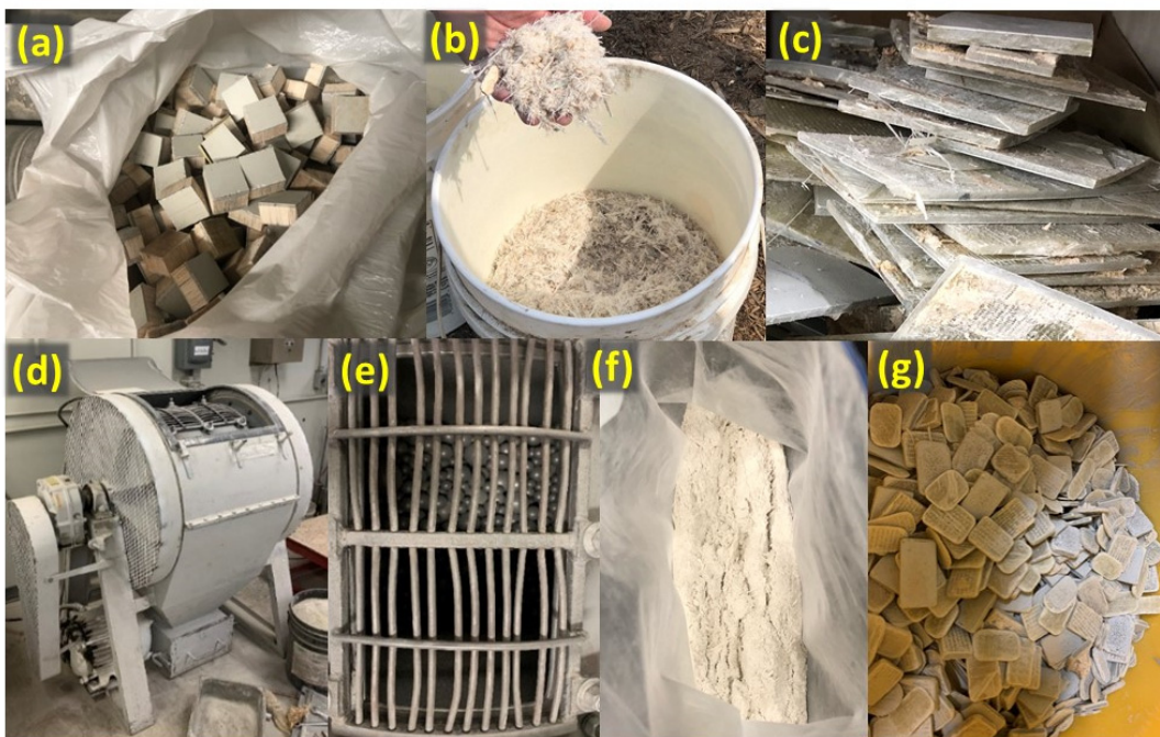
Figure 2. Preparation of waste glass fiber-reinforced polymer (GFRP) material from wind-turbine blades (WWTB): (a) raw material cut into cubes for incorporation in concrete as aggregates, (b) fiber extracted from ground WWTB-GFRP, (c) removal of wooden content (for powder preparation), (d–f) preparation of WWTB-GFRP powder, and (g) wooden content removed (aggregates).
