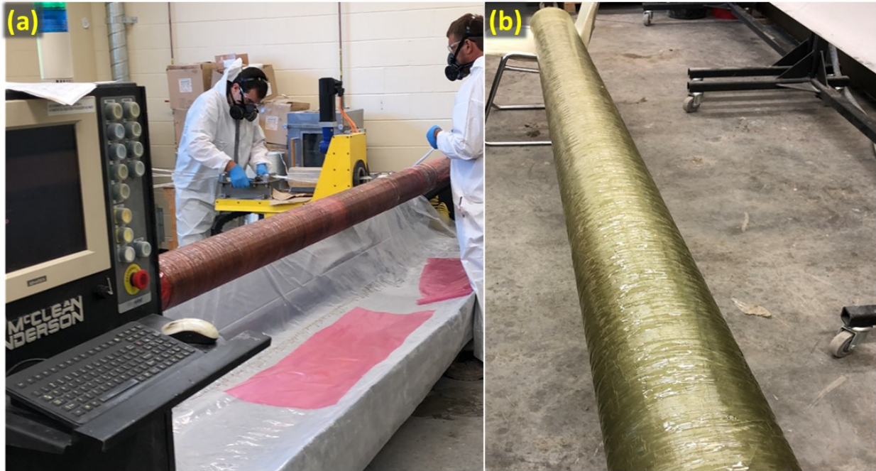
Figure 4. Fabrication of concrete-filled fibre-reinforced polymer (FRP) tubes (CFFTs): (a) filament winding setup, and (b) Final GFRP tube.
