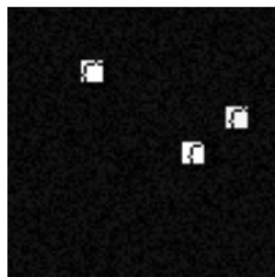
Figure 3. Synthetic frame sequence; Frame 40. The white squares correspond to the ground truth objects moving, while the dark curve inside the squares gives the estimated object outline by applying tracking using a Gaussian kernel with variance in the range [0.001, 1].
