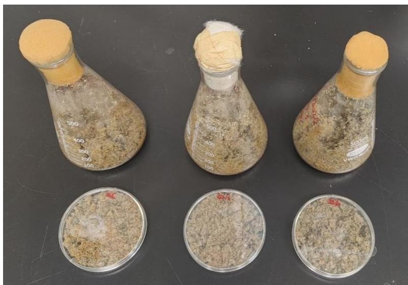
Figure 4. Solid state fermentation with P. chrysosporium on corn maize residues and black spruce chips in flasks and petri dishes.
