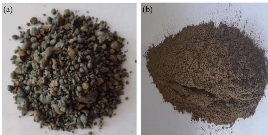
Figure 2. Nickel slag (a) before grinding and (b) after grinding and passing through a No. 400 sieve.
