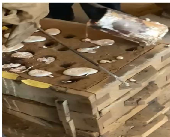
Figure 4. Sand mould with the composites.
