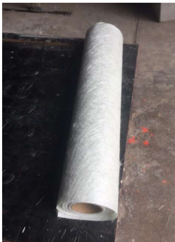
Figure 2. Glass chopped strand mat (GCSM) fiber.
