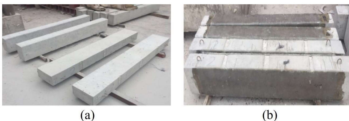
Figure 4. RC shallow beams: (a) before GCSM strengthening and (b) GCSM strengthening.
