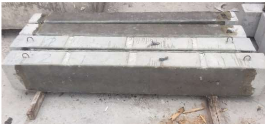
Figure 9. GCSM sheet strengthening of RC beams.
