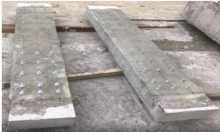
Figure 10. MBA system for strengthened beams.
