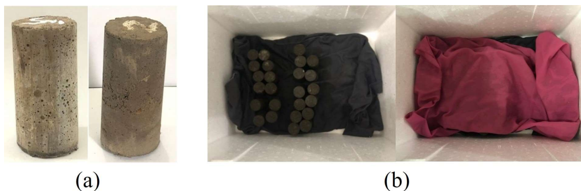
Figure 2. Metakaolin-based geopolymer using bemban fiber mortar. (a) specimen and (b) curing procedure.
