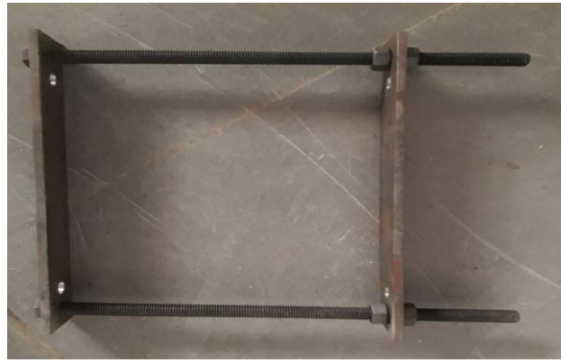
Figure 4. Frame construction for holding wire for reinforcing with Al matrix.
