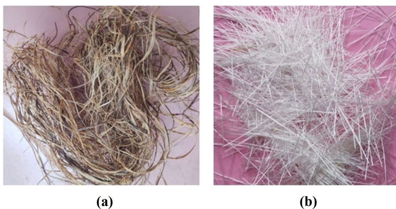
Figure 1. Digital images of (a) screw pine fibers and (b) E-glass fibers.
