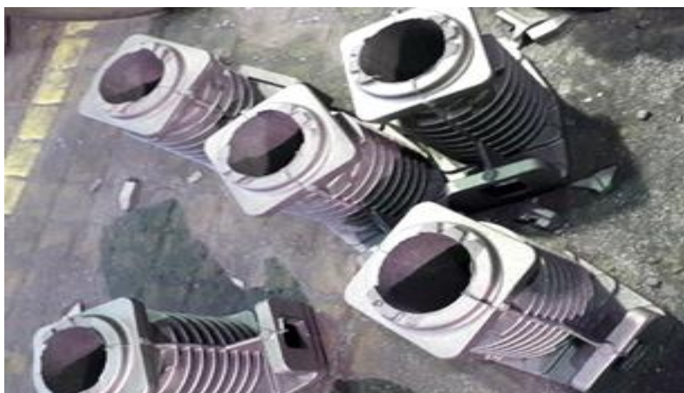
Figure 5. Casting “cylinder”, obtained from the proposed composition of the mixture.
