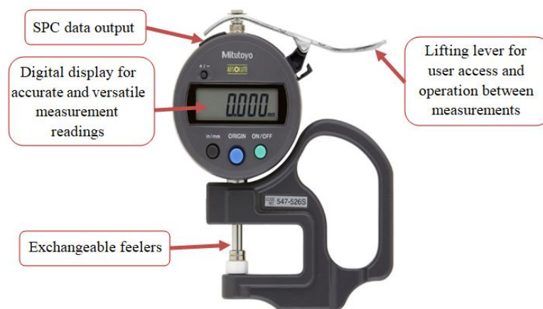
Figure 1. Mitutoyo ABS digital thickness gauge used for the measurement of chip thickness.
