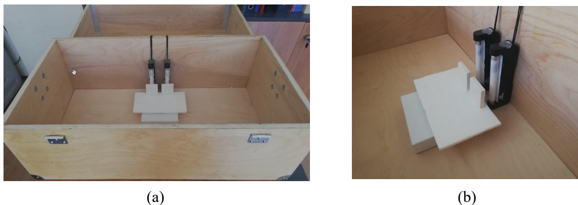
Figure 3. Handmade photocatalytic apparatus for blocks.
