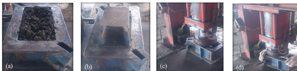
Figure 4. Pressing work step description: (a) put the aggregates into the mold, (b) close mold with plate, (c) press hydraulic aggregates in the mold, and (d) separate mold and aggregates.
