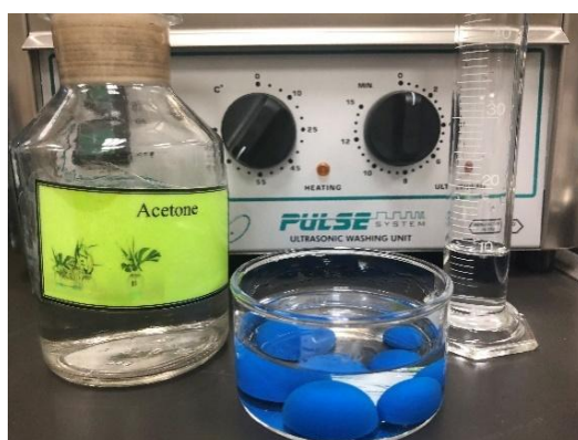
Figure 5. Chemical treatment bath with 80% acetone and 20% deionized water.
