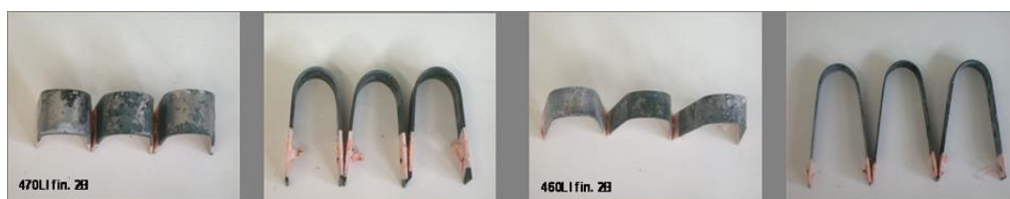
Figure 6. U-bend samples of 460LI and 470LI after 500 h of immersion in \text{MgCl}_2 .
