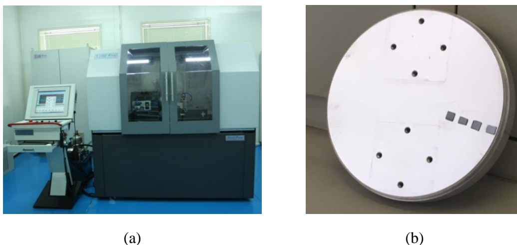
Figure 1. Configuration of diamond turning of monocrystalline Si. (a) Experimental setup; (b) clamping apparatus.
