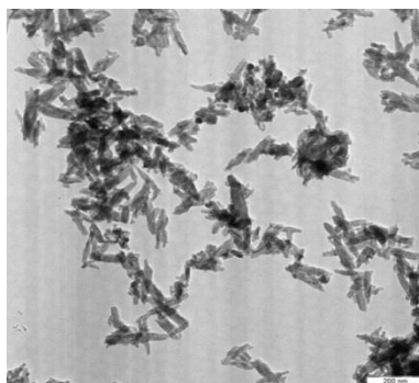
Figure 2. TEM micrograph of nanoZrO 2 -SiO 2 -HA at low magnification (40000×)
