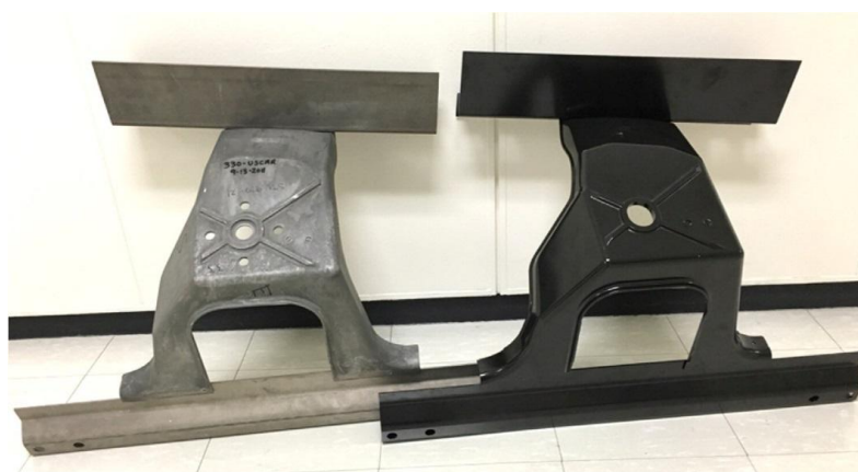
Figure 11. Example of joined Mg structures: An all Mg structure joined using FSW (left); a multi-material structure with a steel upper rail and Al lower rail attached to a Mg shock tower (Right) [7].
