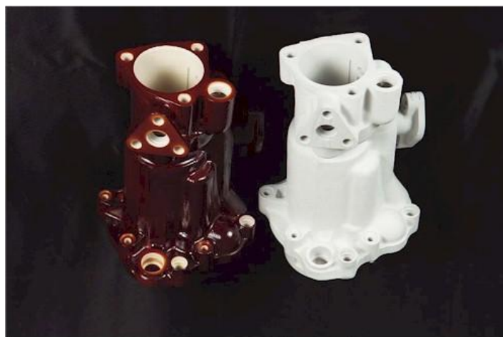
Figure 7. Mg oil pump housing with Tagnite coating: Tagnite with paint (left); Tagnite alone (right) [71].
