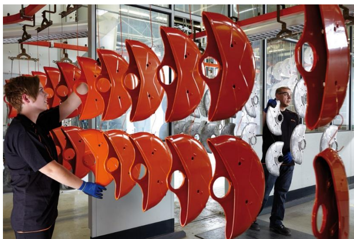
Figure 8. Mg engine parts using powder coating which shows perfect appearance and excellent protection [79].
