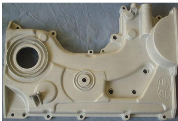
Figure 5. IMR phosphate conversion coating used on Mg alloy hood shield by FAW [51].
