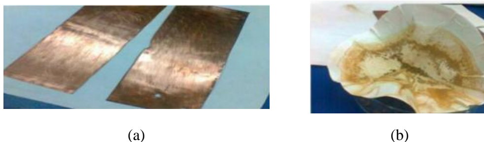
Figure 2. (a) The anode and cathode of electrolysis and (b) the resulting copper oxide powder.
