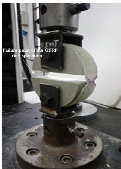
Figure 12. Typical failure pattern observed in E- and S-GFRP rings during testing.
