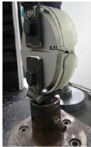
Figure 4. Split-disk fixture fabricated by using CNC Lathe machine.
