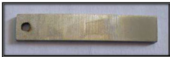
Figure 10. ZnO thin films after 390 h salt spray test.
