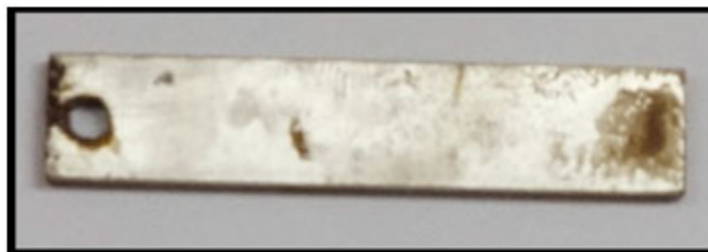
Figure 9. Bare SS 304L after 390 h salt spray test.
