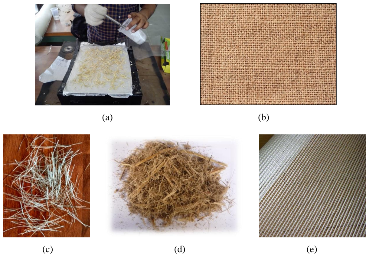
Figure 1. Schematic representation of (a) Hand lay-up technique (b) Jute fiber sheet (c) Chopped glass fiber (d) Bagasse fiber (e) Glass fiber mat.
