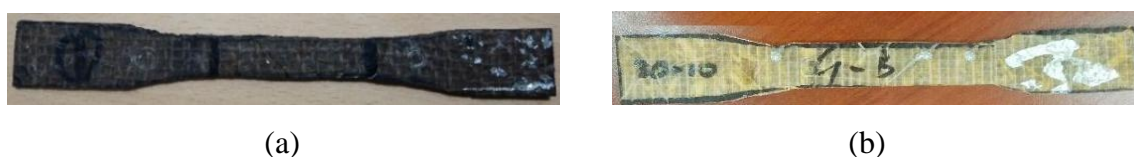
Figure 3. Tensile test specimens (a) jute-glass/epoxy, (b) glass-bagasse/epoxy.
