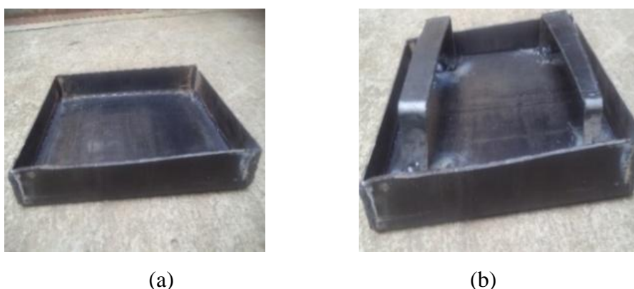
Figure 2. (a) Mold plate, (b) mold plate with cover frame.
