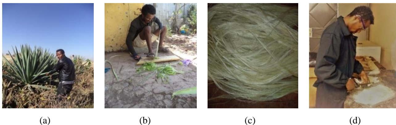
Figure 1. (a) Harvesting the sisal plant, (b) extraction process, (c) the extracted fiber, (d) chopping sisal fiber.
