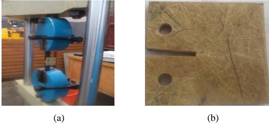
Figure 7. (a) Typical CT specimen under compact tension test using UTM machine in AAIT lab, (b) sisal fiber reinforced epoxy composites after compact tension test.
