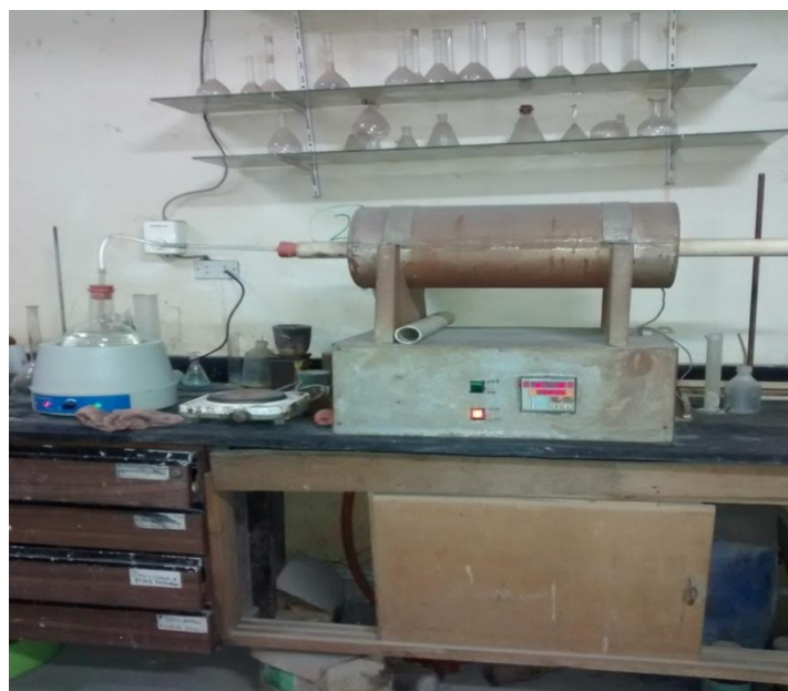
Figure 2. A Photograph of the experimental rig used to activate carbon.
