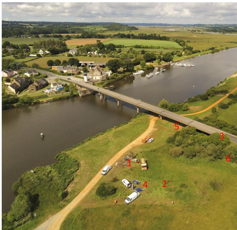
Figure 3. Position of tests at Cran site: (1) different sampling equipment, (2) self-boring pressuremeter, (3) embankment monitoring, (4) shallow foundation tests, (5) piles tests, (6) sampling zone.
