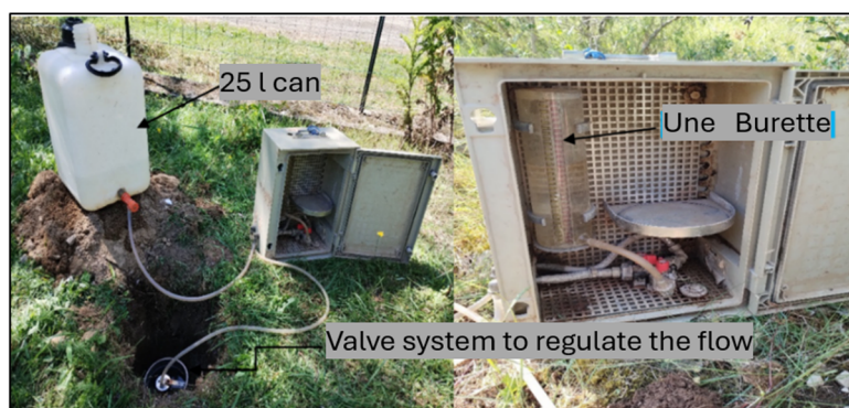
Figure 13. Schematic diagram of Porchet-type permeability test.
