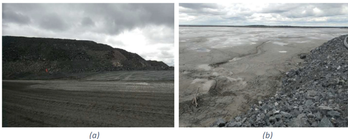
Figure 1. Storage of solid mining waste at the Canadian Malartic mine [1]: (a) waste rock piles, (b) tailings area.
