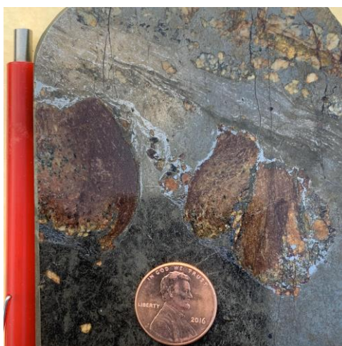
Figure 5. Light grey-silvery telluride fine veinlets in massive dark colored pyrrhotite + dolomite (brownish white) and surrounding the host rock breccia from of the deposit.
