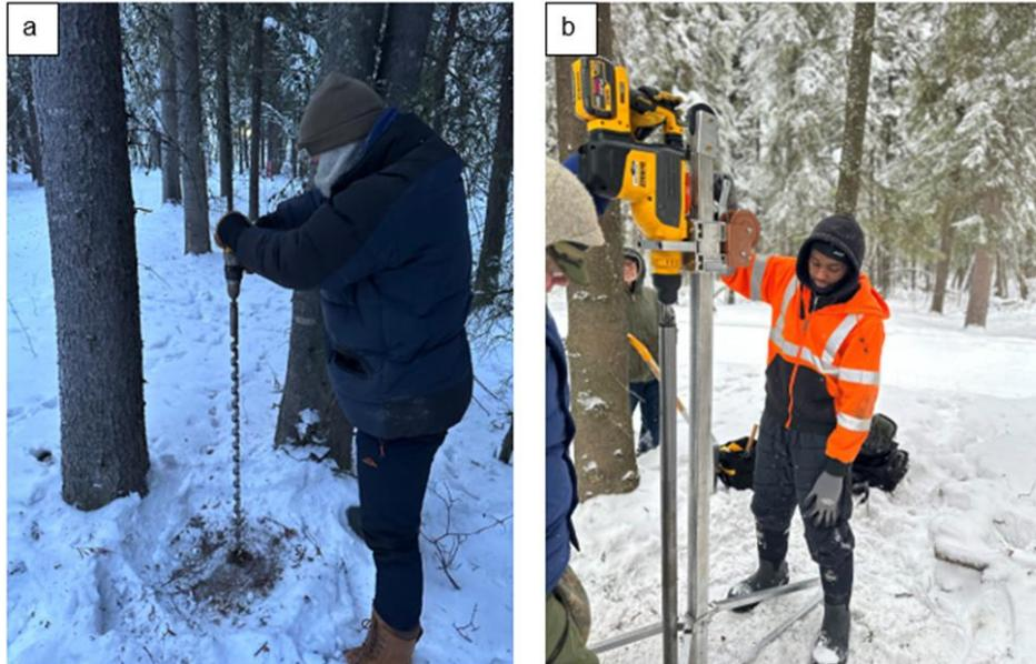
**Figure 3.** Borehole drilling along Profile 4: a) hand-held drill (January 15, 2023) and b) core drilling (March 9, 2023).
