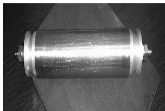
Figure 3. Sand chamber made of steel.
