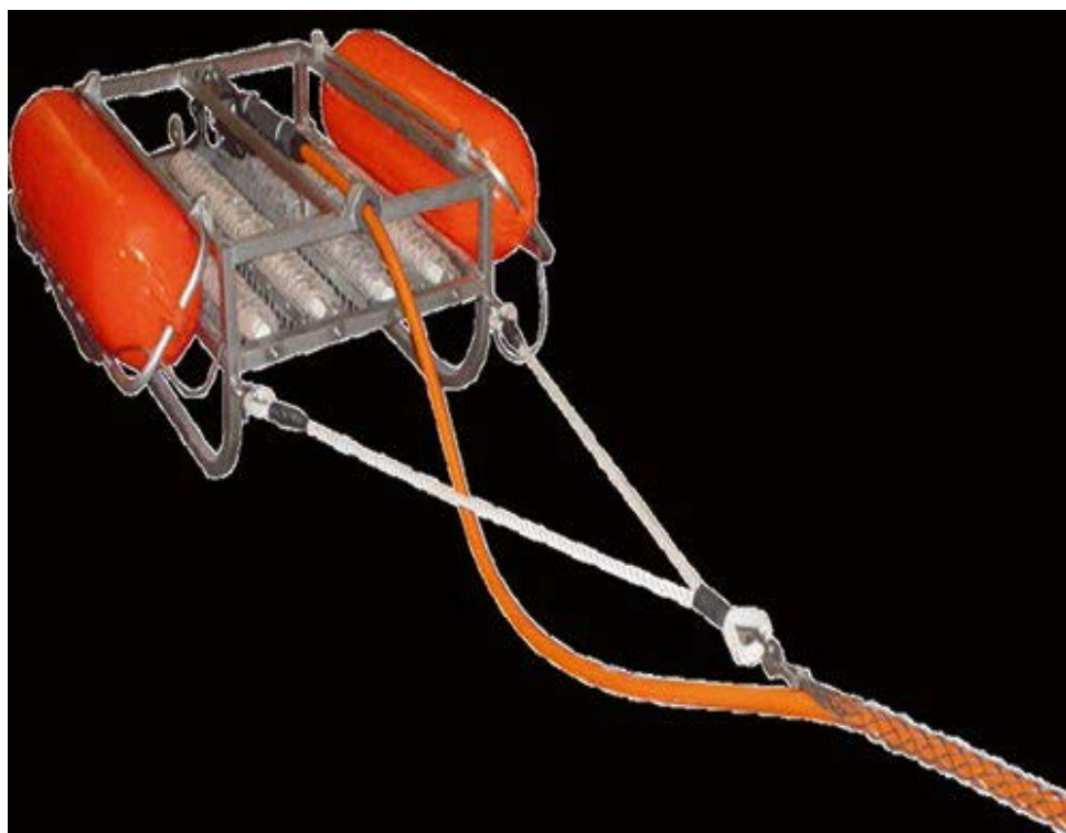
Figure 7. Source of seismo-acoustic waves—Sparker. Marine Multi-Tip Sparker System [26].
