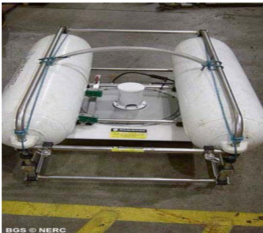
Figure 6. Source of seismo-acoustic waves—Boomer [25].
