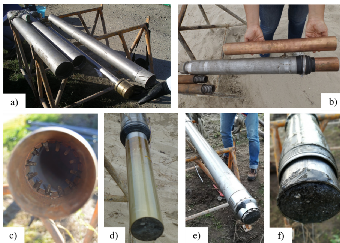
Figure 9. Collection of the high-quality samples: a) GP-S before assembling; b) D&M sampler before collection of samples; c) Mazier sampler; d) D&M sampler after sample collection; e) and f) GP-S sampler after sample collection.
