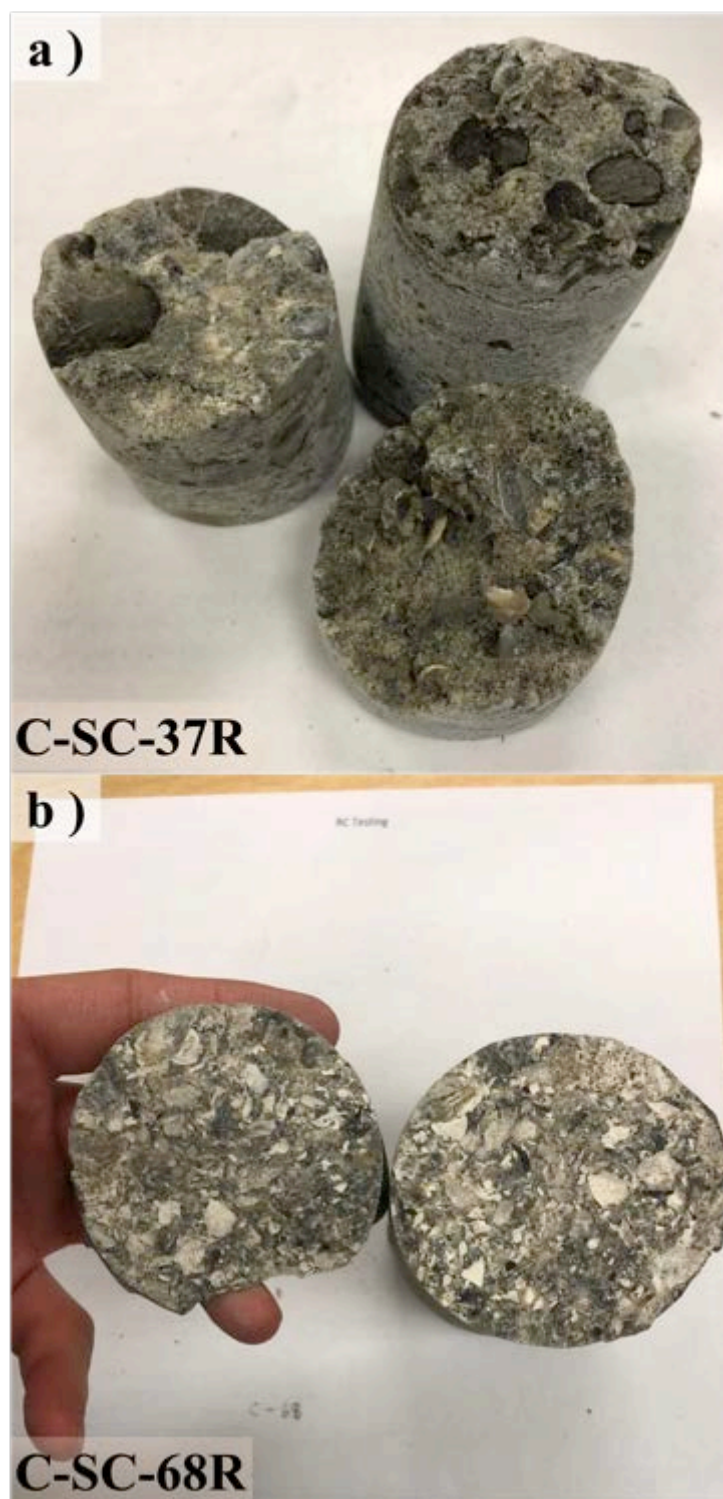
Figure 11. Calcareous Sand/Sandstone Samples from Site A at a Depth of: a) 59–61 m, and b) 137–139 m.
