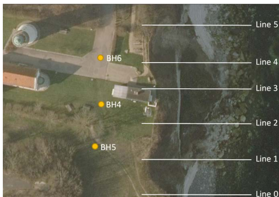
Figure 4. Layout of the present investigations (including boreholes BH4–BH6 and face logging lines 0–5).
