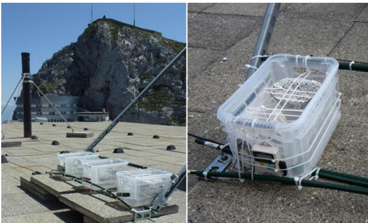
Figure 1. Left: Experimental setting of exposed rock samples located on the roof of the hotel building on top of Mount Pilatus (Central Switzerland). Right: a pair of freshly broken mirror-faced granite surfaces is visible in the box. One surface was facing upwards (back) and the other downwards (front) to determine the influence of atmospheric deposition. A humidity and temperature sensor was mounted at the front of the box.
