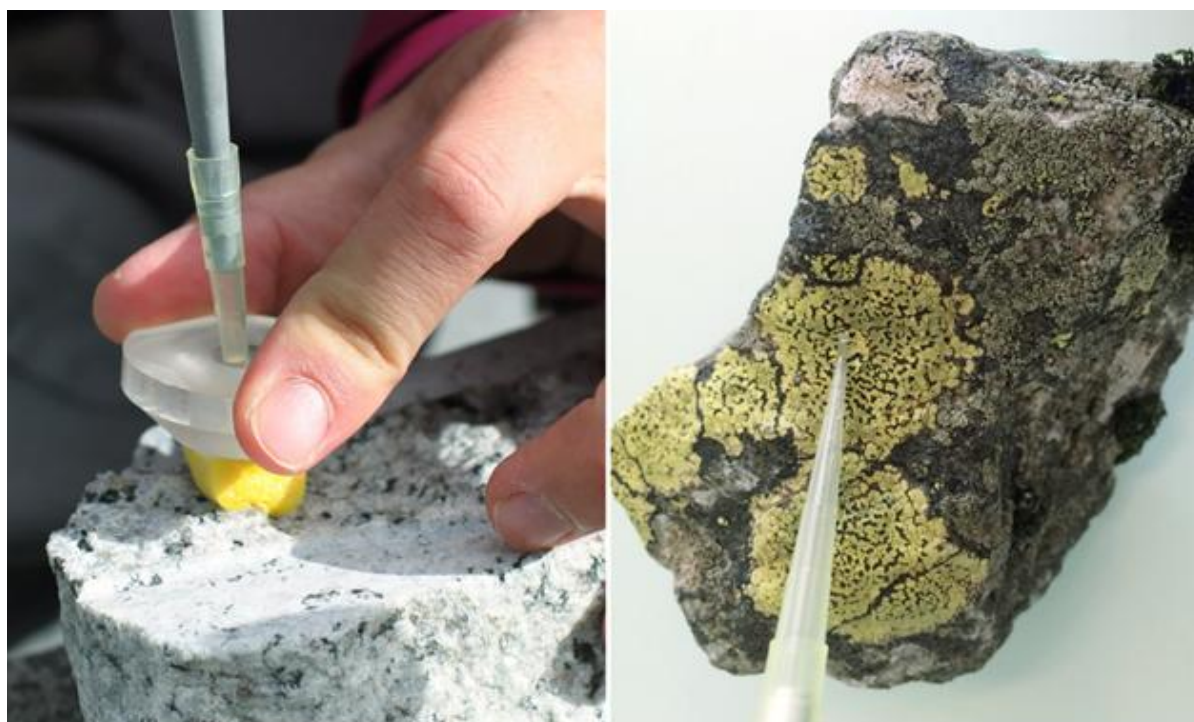
Figure 2. Left: Applying the DoR method on a freshly broken rock surface with the confining rubber foam ring (yellow) pressed on by a plastic ring (colorless, opaque). Right: Applying the DoR method on R. geographicum growing on a granite specimen. Note that the drop at the pipette tip remains intact due to the hydrophobic nature of the lichen's surface.
