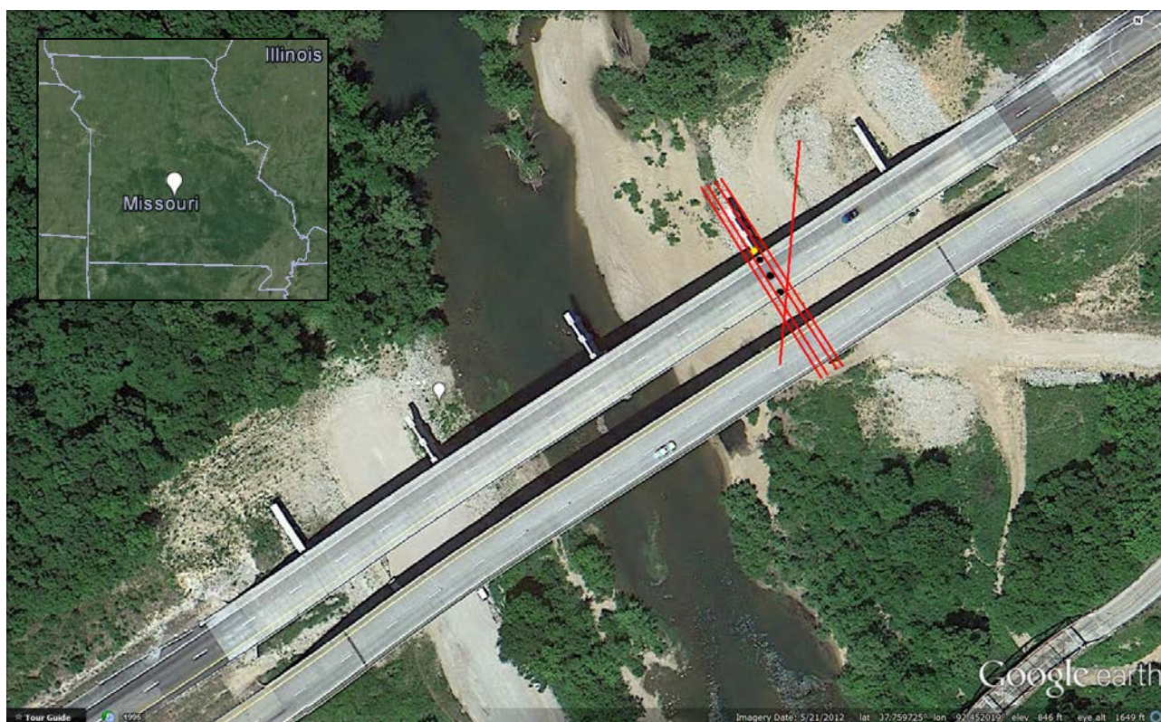
Figure 1. Aerial photograph of the Gasconade River project site (Google Earth) in Central Missouri with superposed ERT traverses (marked as red lines). The temporary structure is located northwest of the Gasconade westbound lane bridge. The black dots depict locations of the existing columns, yellow — the proposed column.
