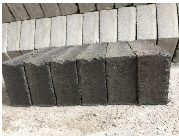
Figure 6. Paving blocks from incinerator medical waste.
