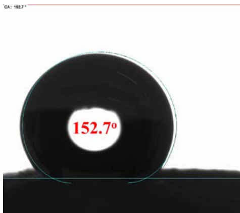
Figure 6. The water contact angle on the surface of RP aerogels coated with MTMS.
