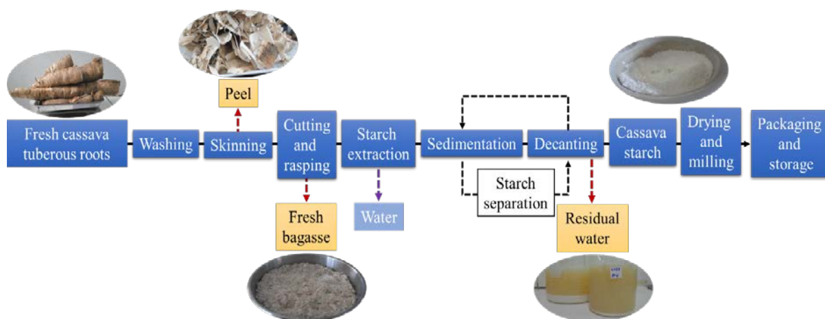
Figure 5. Diagram of the cassava starch extraction process from the wet pulp.
