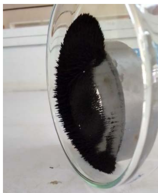
Figure 1. Synthesis results of Fe 3 O 4 nanomagnetite applied with magnet external.
