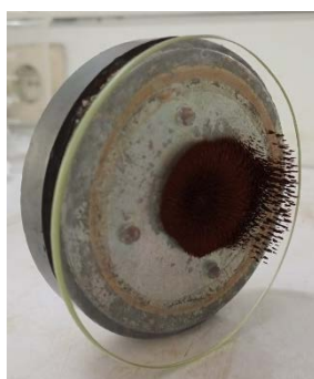
Figure 2. Fe 3 O 4 /SiO 2 -AO nanocomposite applied in an external magnetic field.
