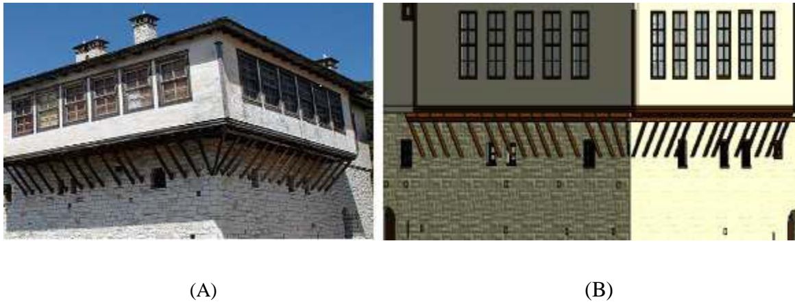
Figure 3. Structural framing elements of the museum. (A) Real building, (B) BIM model.
