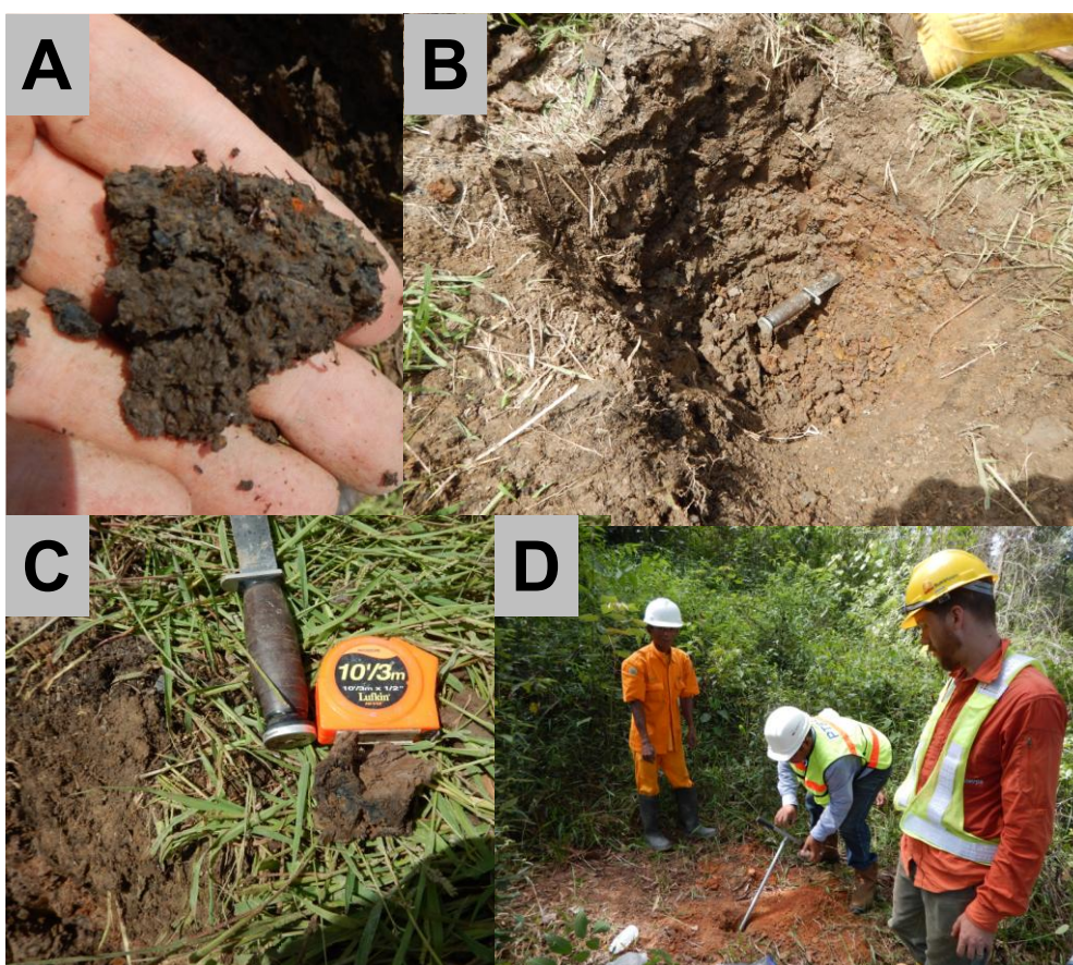
Figure 3. Photographs showing the general characteristics of the reclaimed mine soils. Panels A & C Show a ped with organic matter coating at the Agroforestry Tupak – Bloc 1 site (3-month-old). Panel B shows an example characterization pit. The gradation from the more organic-rich near-surface soil to redder mineral soil can be observed with depth. Panel D highlights the much redder soils and lack of surface organic material at the Banko Barat 3 site.
