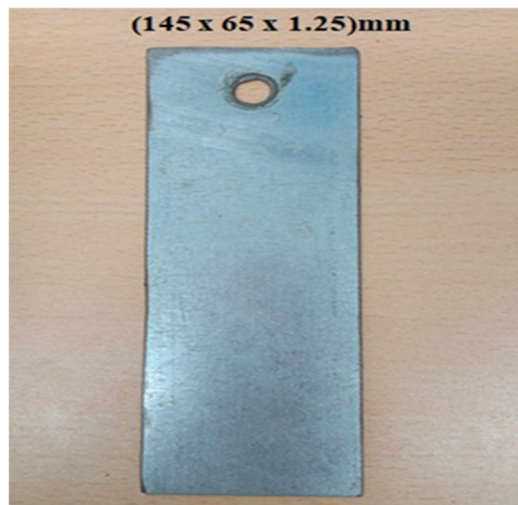
Figure 22. Ideal steel plate: length = 145 mm, width = 65 mm, thickness = 1.25 mm.
