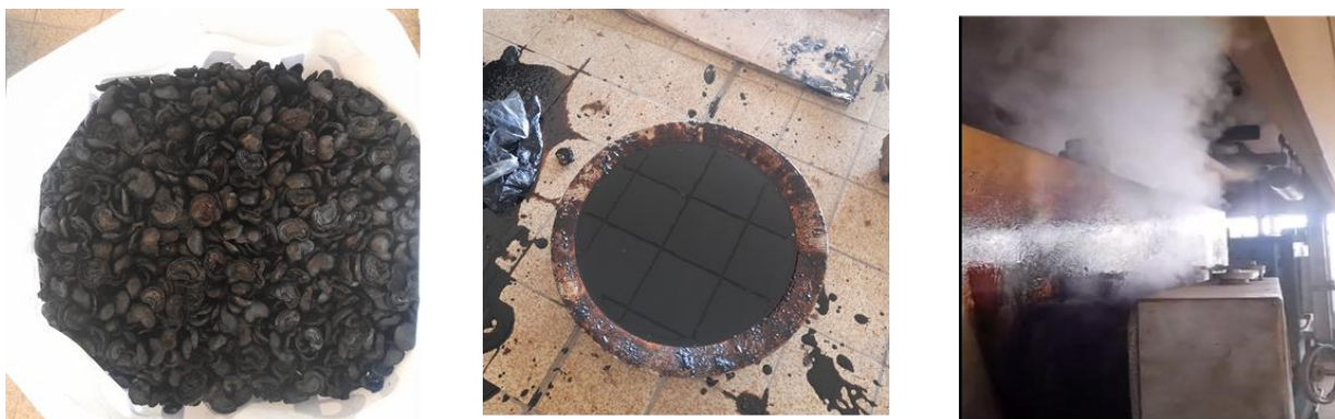
Figure 3. Products of the heat treatment process (biochar, bio-oil and smoke).
