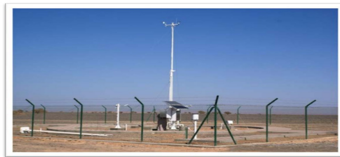
Figure 11. Sun Tracker with pyr heliometer installed at Nizwa-Manah [Nizwa-Manah Environmental Station].
