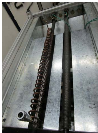
Figure 3. Laboratory system for pulsed heat pipes and fin-equipped tubes.
