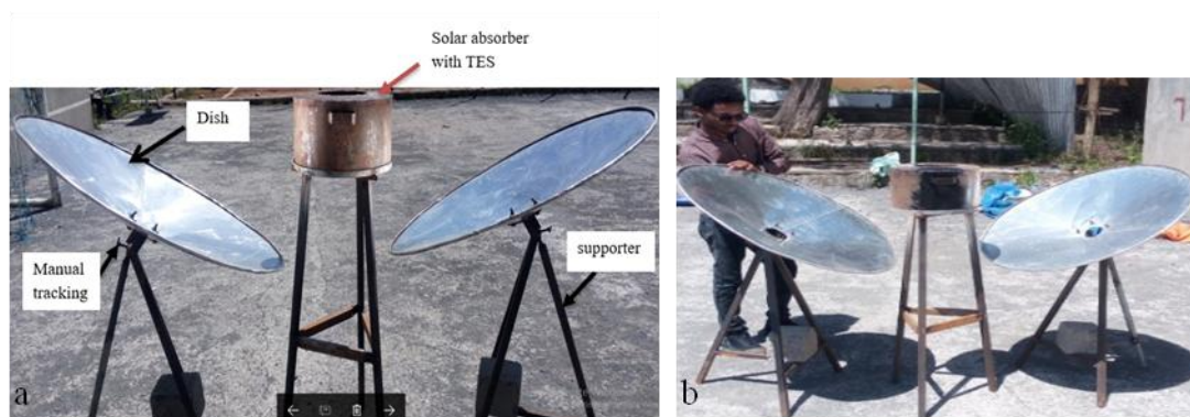
Figure 4. Experimental setup (Photograph). a. Over all system; b. manual tracking of parabolic solar collector.
