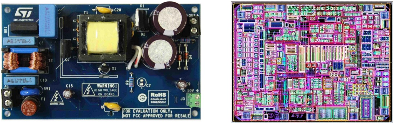
Figure 9. LED driver prototype (left); control IC layout (right).
