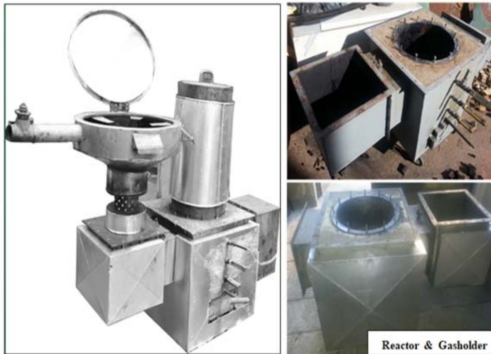
Figure 2. Injera baking biomass gasifier stove and reactor under construction.
